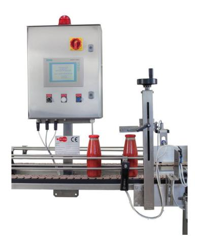
**Speed**: up to 600 caps per minute (the manufacturer confirms the maximum feeding speed according to the cap/jar type).
